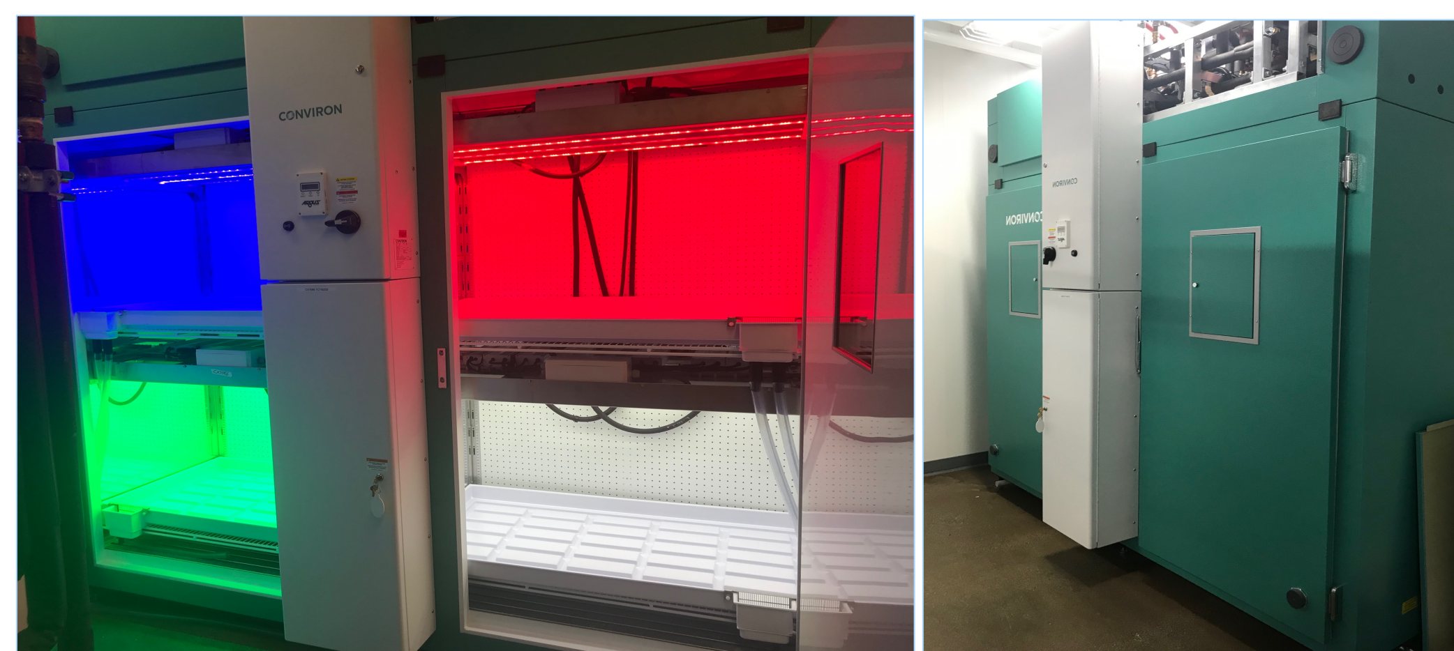
Figure 1. Four different lighting spectrums set up in a two tiered modified PGC Flex chamber.
